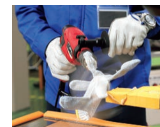
回転刃物手袋巻き込み体感 Demonstration of a Glove Catching in a Rotating Tool
