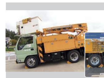
高所作業車逸走防止装置 Aerial Work Platform Vehicle Movement Prevention Device
