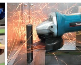
研削といしはじかれ体感 Grinding Wheel Kickback Demonstration
